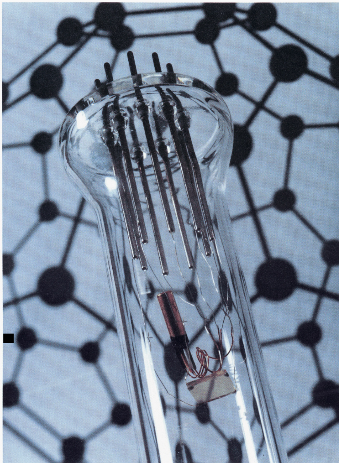
Figure 3. Apparatus for measuring conductivities of doped fullerene films at low temperatures. The amber C_{60} film is on a glass substrate above an internal thermometer.
